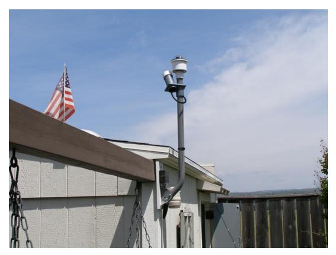
Choose a location for mounting the camera that is as high as possible to avoid obstructions near the horizons. An adjustable mask is incorporated into the camera to block unwanted light on the horizon as needed. The camera can be mounted on a standard 1.66'' diameter satellite dish mount such as the <u>Winegard DS3000</u> or on a standard 1-1/4'' diameter PVC pipe. Orient the marks on the camera housing so that they are pointing to North if desired.
